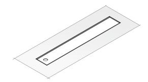
To remove the strip place an allen in the chuck of a drill and use it to peel the tearout strip away from the housing.
