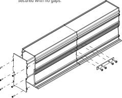
In-Line: If product is to be installed in-line the flange will be supplied separately. Use the screws provided to attach them to the outside of the in-line length.
