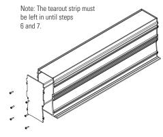
Multiple - Use the connection kit provided. The two sections must be secured with no gaps.
